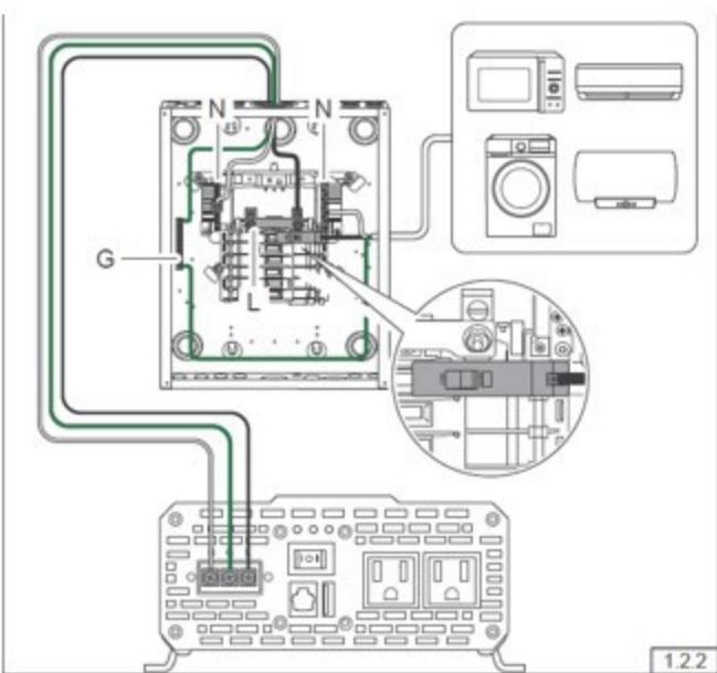
You can also permanently connect the AC output from the AC hardwire terminal through the AC knockout into a load sub-panel or additional AC outlets powered by the 1000W/2000W/3000W inverter. From left to right, the terminal block indicates: Live/Hot (L), Neutral (N), and Ground (G).
